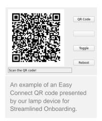
When a user scans the Easy Connect QR code presented by a device (on its display, manual, box, etc.), the Easy Connect Configurator opens a secure Layer 2 channel with the new device. OCF Streamlined Onboarding information is provided during this configuration exchange to facilitate device onboarding after network association is complete.
