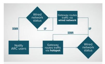
ARC Hotspot detects when a wired network is down and automatically shifts traffic to a cellular hotspot until the wired network is working again.
